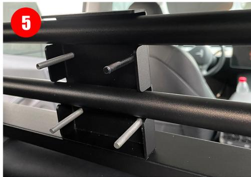
5 Place the cover box with screws on the pet partition above the seat, Please notice the direction of bracket.
