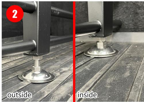
2 Adjust the nut as shown in the diagram, screw the inner base to the bottom, and adjust the outer base so that the inner support bracket can fit snugly against the seat.
