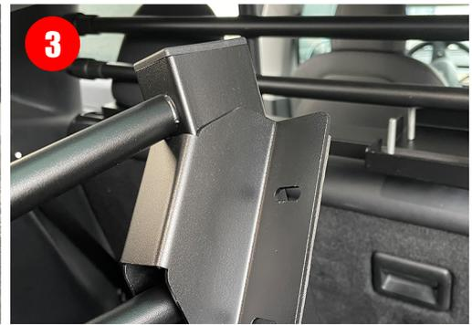
3 Insert the cover box with holes into the gap of the first layer above the bracket, following the illustration
