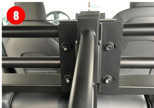
8 Install the washer and screw nut.
